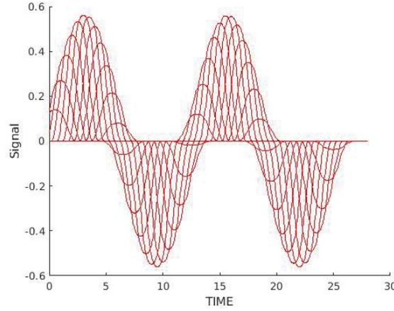
**FIGURE 2.** Formation of signal by individual wavelets. Since only a small number of wavelets overlap, individual antennas in an array can be used repeatedly: the proposed antenna system radiates like a Gatling gun fires bullets: each single antenna at a time with some overlap
